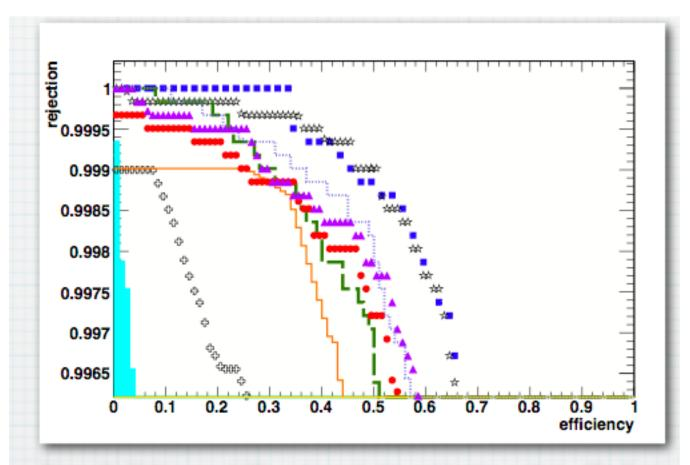
Figure 19: Performance of  $GL_K$  and set of other multivariate methods. The X axis shows the efficiency, and the Y axis the rejection. Blue squares:  $GL_K$ , Open stars: BDT. Short Dashed: PDERS-PCA. Violet triangles: Fisher Discriminant. Red cyrcles: Best performant NN.Green dashed line: Support Vector Machine.Orange solid line: RuleFit. Open crosses: less performant NN. Filled Cyan histogram: FDA-SA
