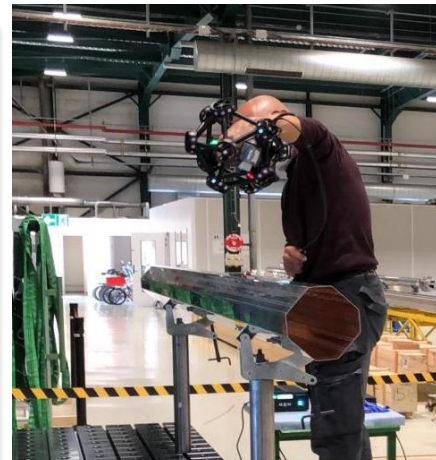
High precision 3D scanner metrology
