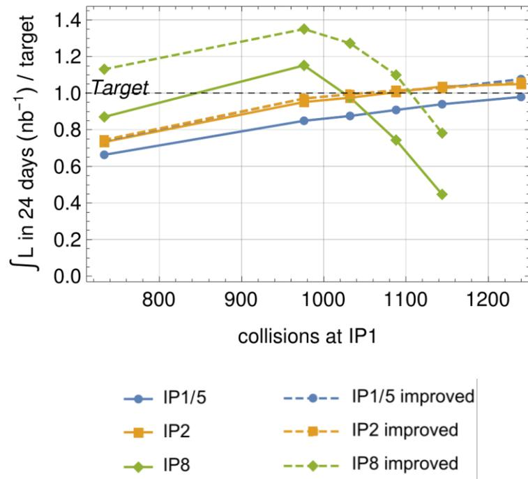
*Example of improved configuration: 100 urad net crossing at all IPs,  $\beta^*=0.45$  m at IP1/2/5,  $\beta^*=1$  m at IP8: reach target with 50% OP efficiency*
