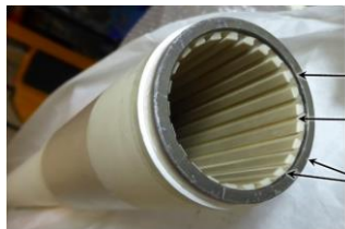
Silver paint Slots for screen conductors Radiused edges
