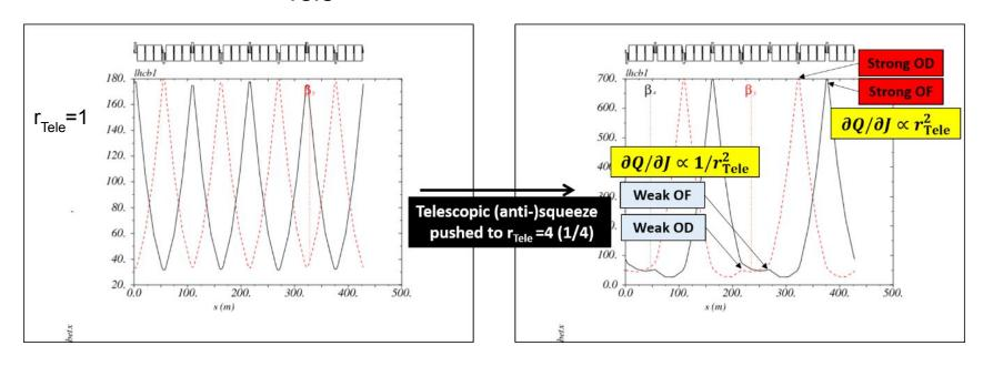
This allows for stronger Landau damping and to keep constant lattice elements between IP and Roman pots in physics. **2023 optics to be tested in 2022 MDs**
