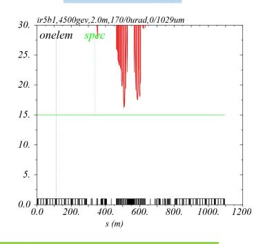
The anti-telescope (@  $\beta^*$  = 2 m) shall be deployed at **E**  $\geq$  **4.5 TeV**, limiting the tele-index reach to about  $\mathbf{r}_{\mathsf{Tele}} \sim \mathbf{0.5}$  **EoR** (@6.5 TeV)
