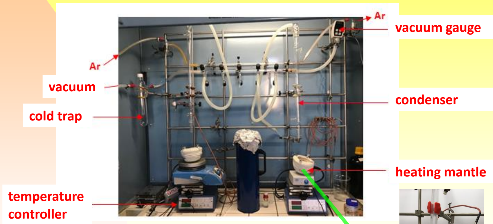
Schlenk line installed at the FNSPE CTU
