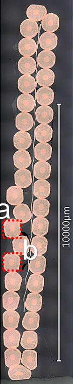
Filaments (belonging to different strands) are affected by cracks in the SC phase
