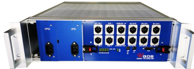
Latest version of the UQDS HL-LHC quench detection system
