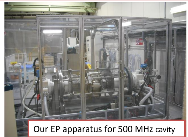
Horizontally rotating EP system developed for TRISTAN SC cavities
