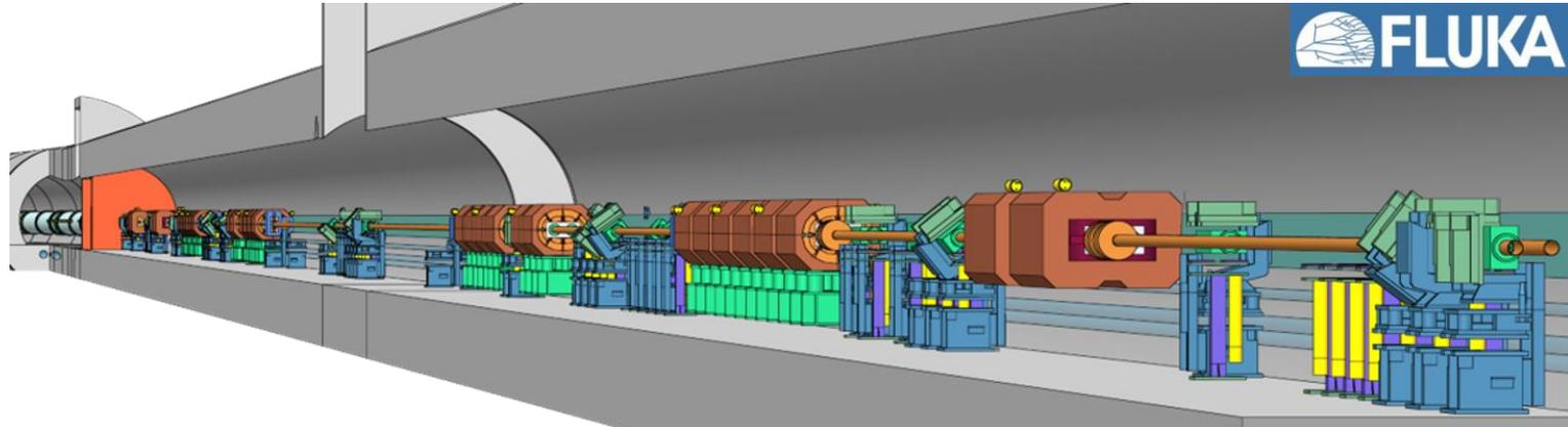
Collimation system in IR7 intercept particles with large betatron oscillation amplitudes
