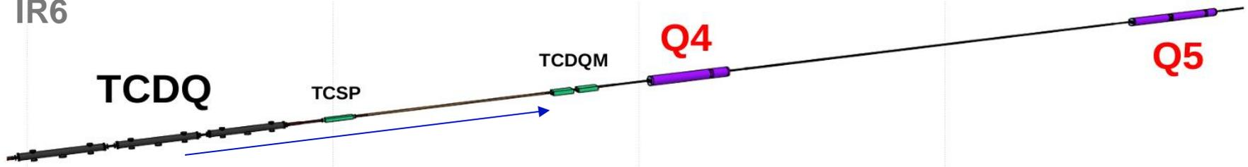
TCDQ/TCSP protect magnets in case of asynchronous beam dump, but they also intercept a fraction of halo particles scattered out of IR7
