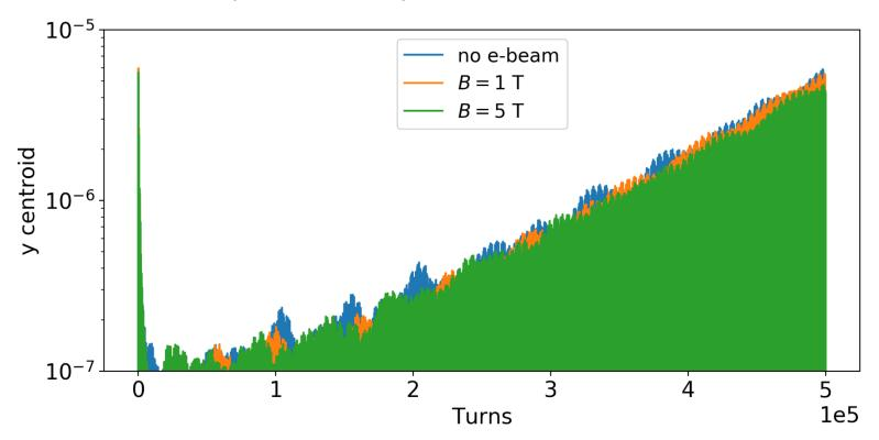
$\Rightarrow$  no strong impact on the most unstable plane (y), even at a lower B field and at a lower x-y tune difference (rise times stay within ~10%).
