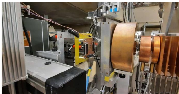
AD7291 ADC test board on the beam line
