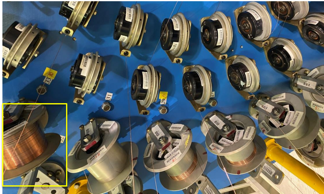
One respool showing excessive residual strand
