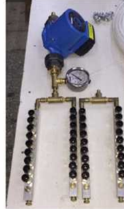
water pump (up to 10 bar)
