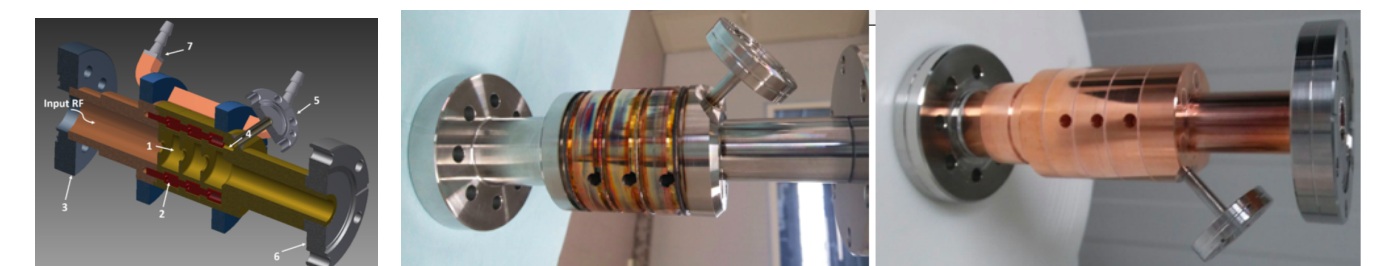
Solid model, one-half of the braze-free 3-cell cavity: 1. High-gradient cells, RF vacuum chamber; 2. Special screws for clamping; 3. Input RF flange 4. secondary vacuum chamber; 5. Vacuum flange for the secondary vacuum chamber; 6. Downstream vacuum flange; 7. Water cooling pipe.
