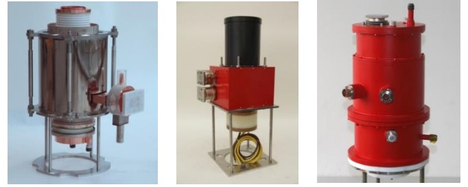
Figure 6. S/C/X band MBK providing \geq 3 MW output power.
