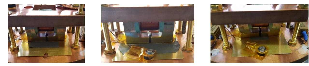
Pb is soft and was cut by a scalpel to determine how the effect of sample size affects the leakage produced. This also allows the field of full flux penetration ( $B_{fp}$ ) to be compared for different sample sizes, and if sample size has any effect.
