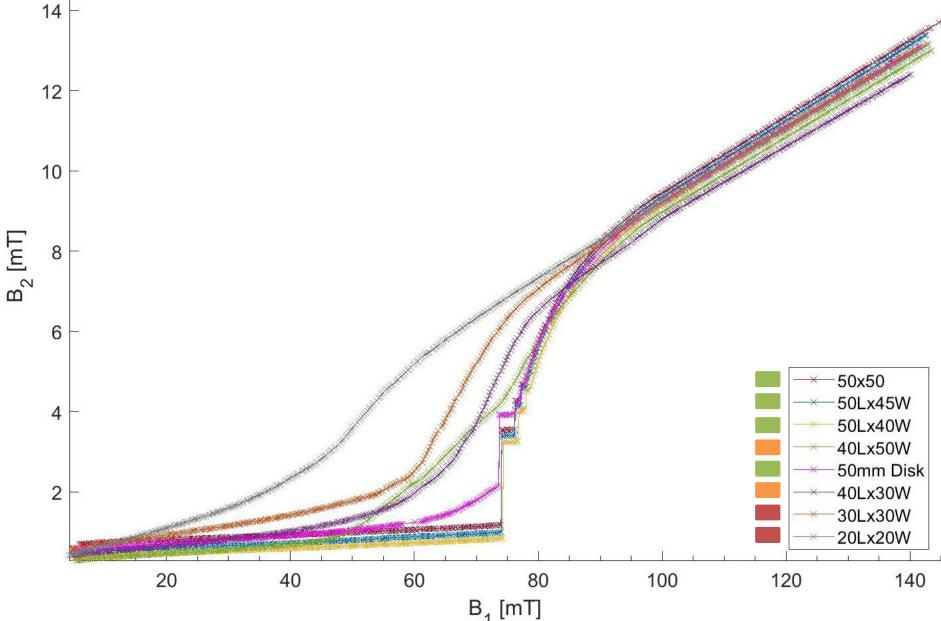
Reducing the sample size creates an increase in the 'Leakage slope'
