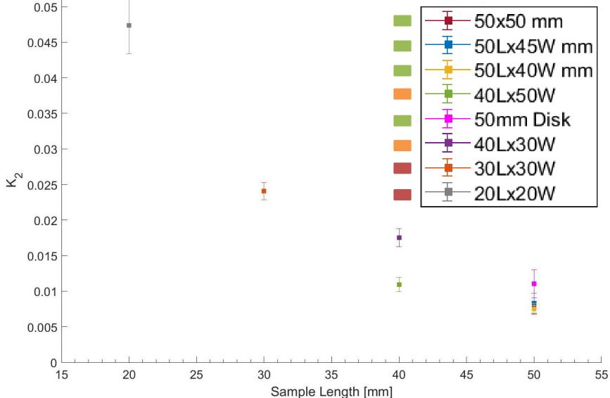
Decreasing the sample size increases the leakage constant, K<sub>2</sub>. Therefore is has been deduced that the length of the sample is important to reduce the leakage.
