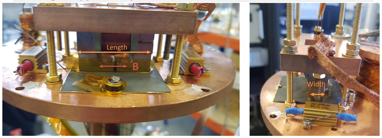
To investigate the effect of geometry a Pb sample (50 × 50 × 0.01 mm) was bought from Goodfellows to determine the effect of sample size. Magnet length = 40 mm Magnet width = 10 mm
