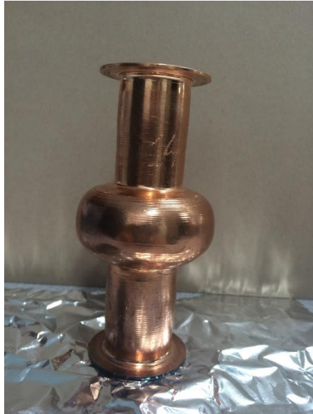
INFN seamless standard elliptical copper cavity
