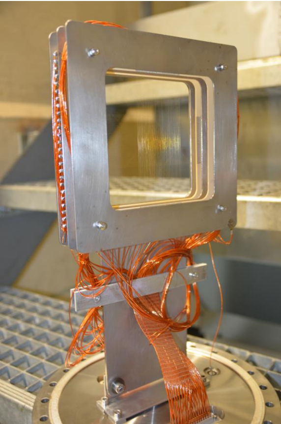
Old style... Kapton wire connected manually
