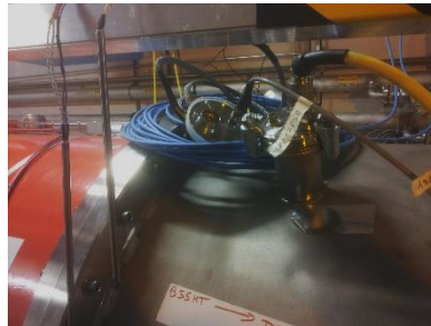
Testing EHBS at P8 (UA87; QYC01&QYC04) crates with long cables (50m&100m) and external load.
