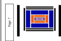
magnet bends the trajectories of particles so can can estimate their momentum; electromagnetic calorimeter picks up electrand photons; the hadronic calorimeter measuractivity from particles made of quarks gluons; and the muon spectrometer tells where muons passed.
