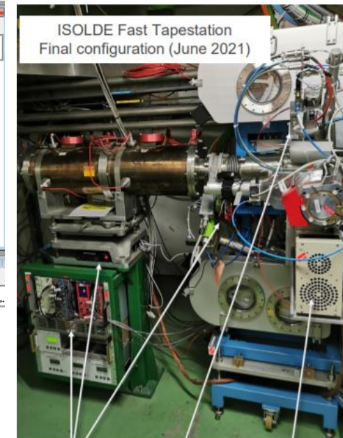
Electronics (HV and preamp power, logic, DAQ) F.CUP P2 position: HPGe \gamma -ray detector
