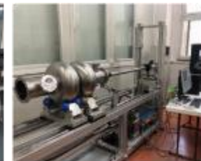
Cavity inspection camera and grinder
