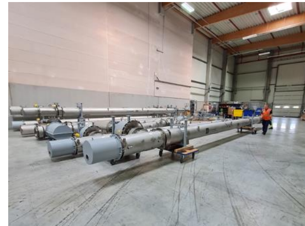
Cryogenic bypass lines (WUST) in storage area
