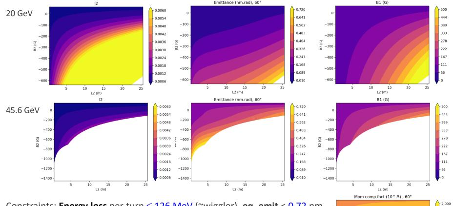
Constraints: **Energy loss** per turn  $\leq$  126 MeV (~wiggler), eq. emit < 0.72 nm
