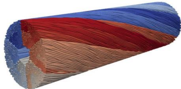
3D FE model of CICC cable based on Multifil [Riccioli 21]
