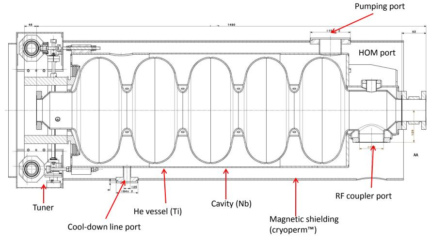
Includes specific features for cryo-module integration (inter-cavity supports, cryogenic feeds, magnetic shielding ...)
