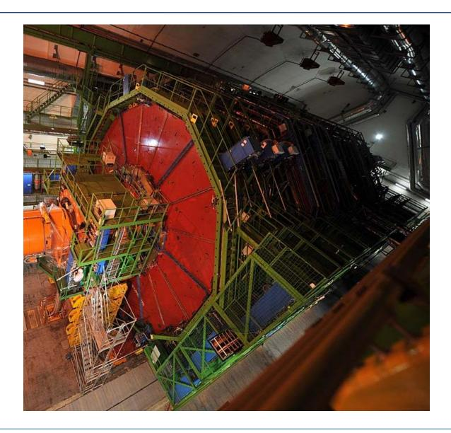
The CMS Muon spectrometer was designed to provide identification, timing and momentum measurements and excellent triggering at LHC conditions (with a nominal luminosity of 10<sup>34</sup> Hz/cm<sup>2</sup>) ...
