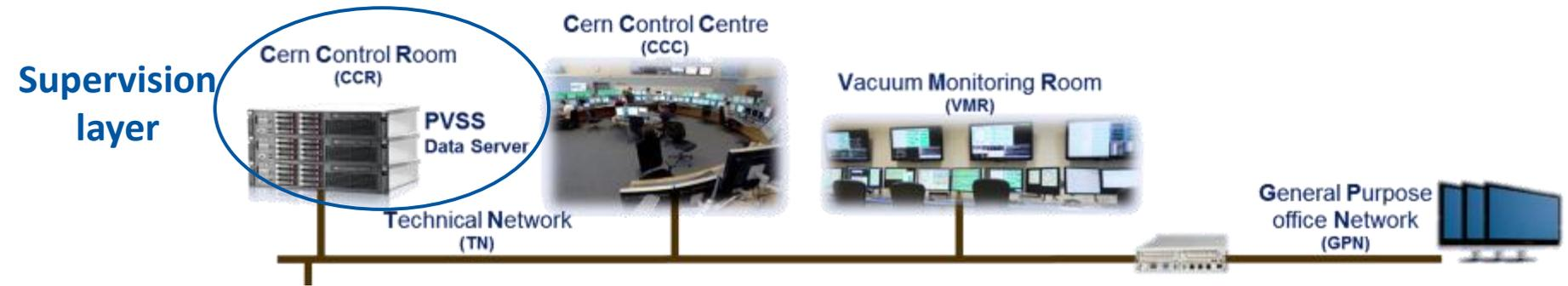
**SCADA** – Supervisory Control And Data Acquisition
