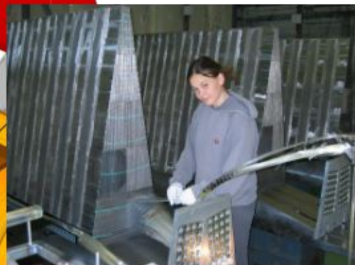
FORWARD CALORIMETER Steel + Quartz fibres ~2,000 Channels
