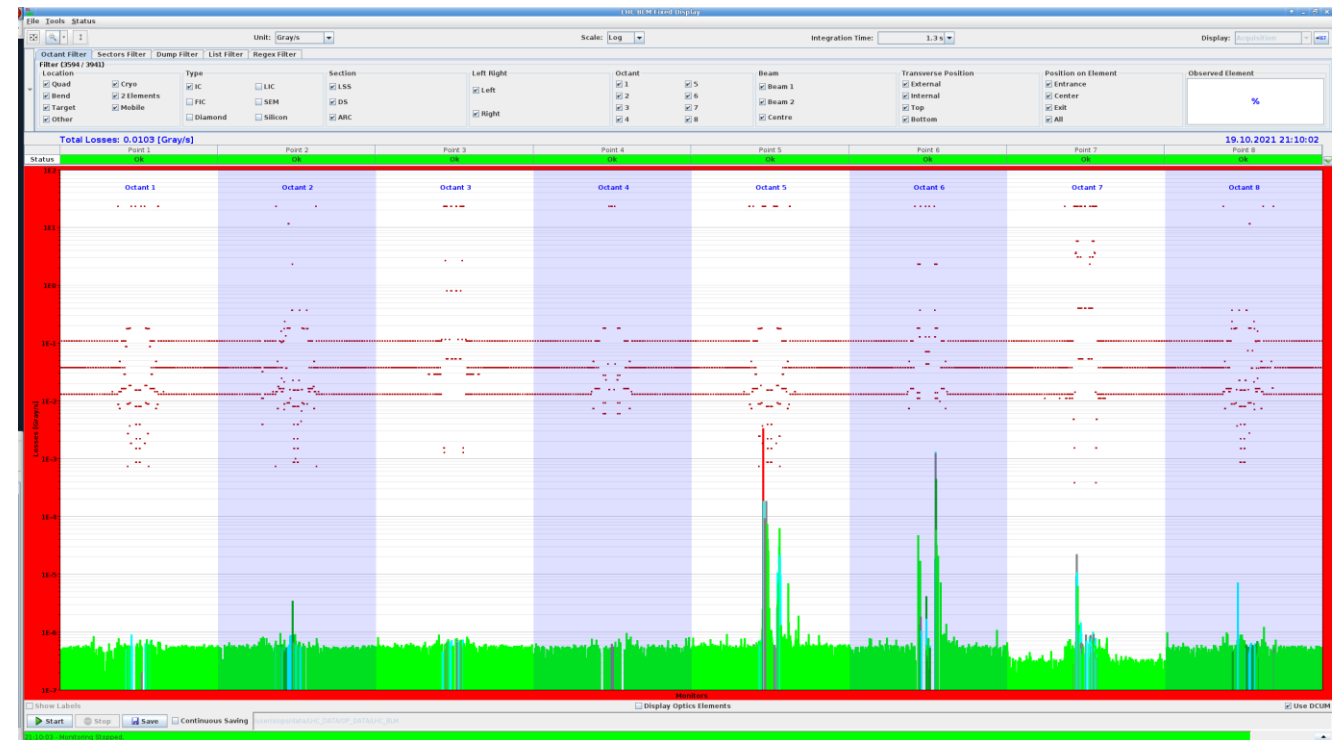
Triggering beam dump in IP5 with B1
