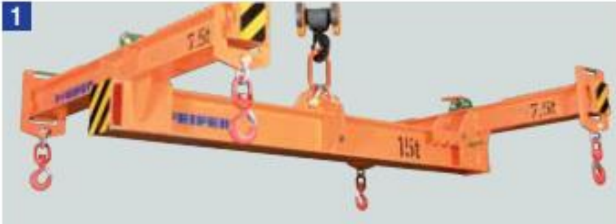
1 Adjustable spreader beam with low construction height Cross beams on top for low heights, cross beams can be used individually. Carrying capacity 15,000 kgs.
