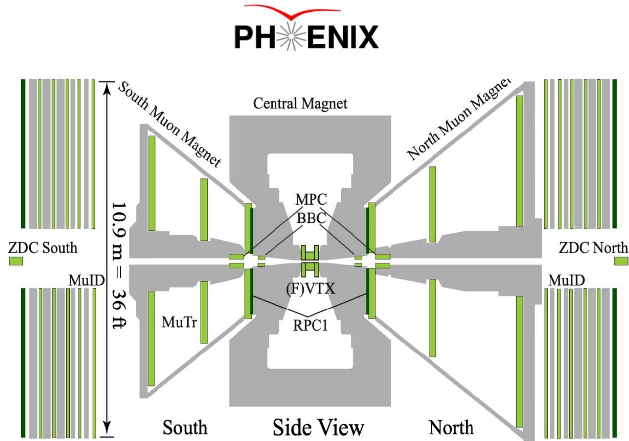
Side view of the PHENIX detector system at RHIC
