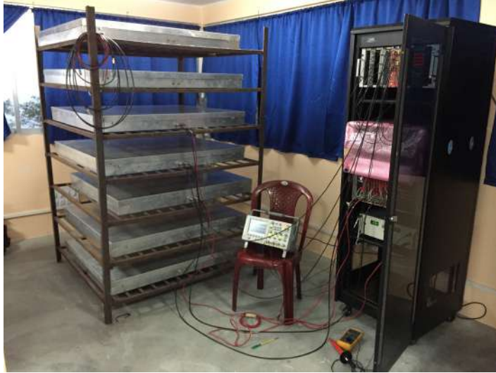
Stack of Scintillator detectors
