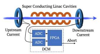
Differential Current Monitor to protect SCL from beam loss damage
