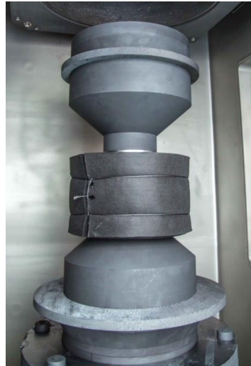
Spark Plasma Sintering (SPS) >25 MPa, >2600 °C
