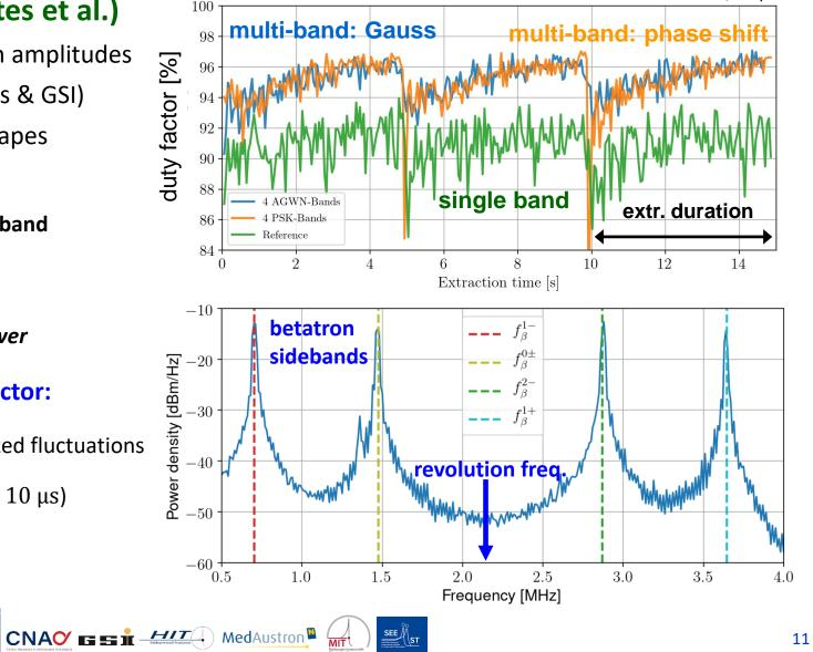
Beam: C<sup>6+</sup> 124 MeV/u, 8e7 ions, tune  $Q_x = 1.68$ Detector: Ionization chamber, 50 µs readout
