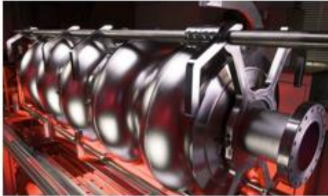
Conventional Niobium cavity
