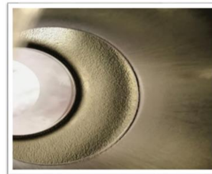
Picture of the inside of a Nb cavity coated with TiN-Al 2 O 3
