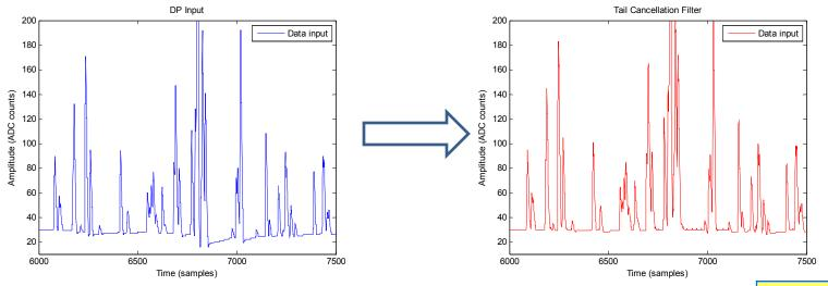
> BC2 example test: rest of the filters are disabled.
