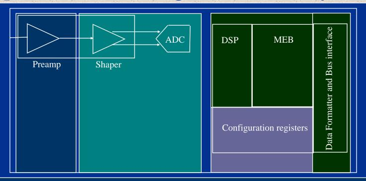
Preamp > Reduce current via bias control, important to maintain a low impedance on the electrode.
