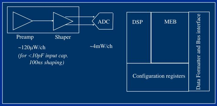
64 channels = Analog power ~ 263mW + Digital power ~ a few hundred mW. Approx. 400-500mW / chip.
