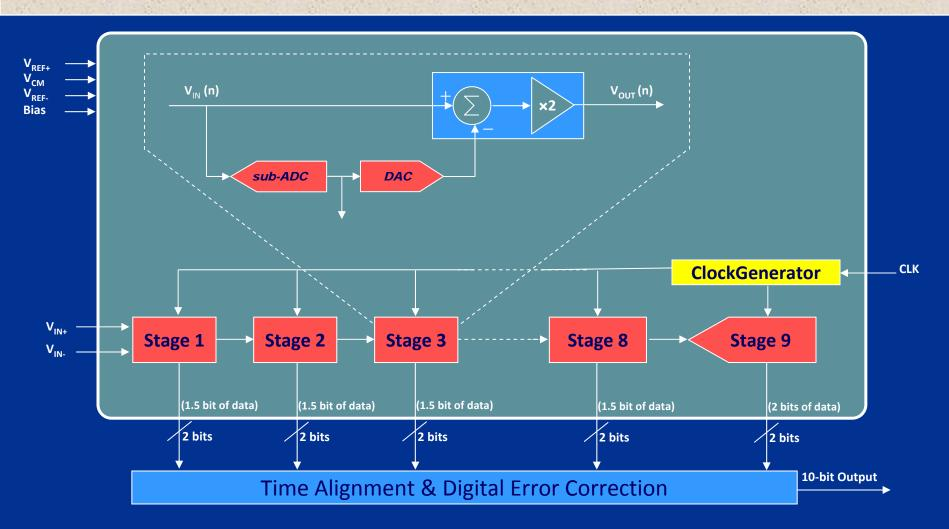
10bit, 40MHz, 1.5V supply, 34mW power, 0.7mm<sup>2</sup> area
