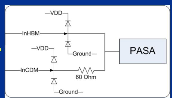
The series resistor adds noise to the input signal.
