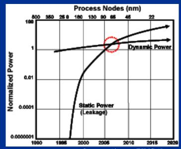
Source: Altera on TSMC 65nm
