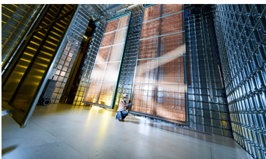
ProtoDUNE: three hundred cubic metre volume prototype Liquid Argon Neutrino Detector being constructed at CERN. (© CERN)
