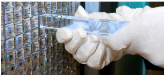
Insertion of lead-tungstate crystals (over three times the density of conventional glasses) into the high granularity electromagnetic calorimeter of the ALICE detector giving percent scale energy measurements. (© CERN)
