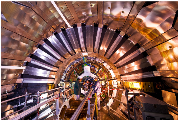
Installation of the CMS Central Tracking Detector with 10 million read-out channels and using silicon detectors covering an area of over 200 m 2 . (© CERN)
