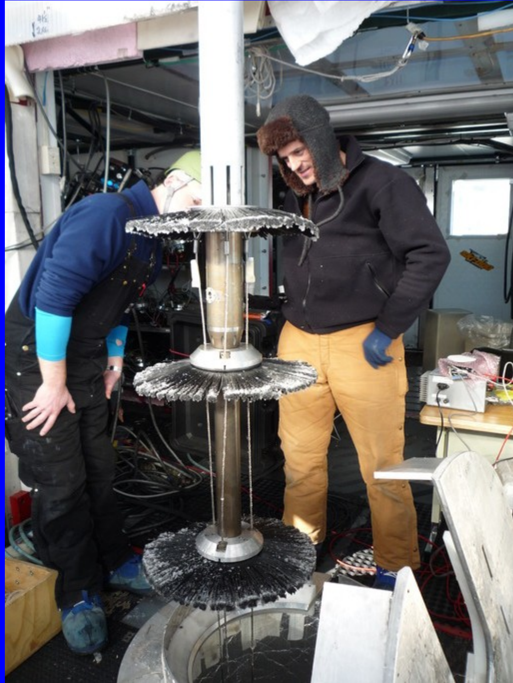
Ryan Bay getting his dust logger ready to deploy in IceCube at South Pole
