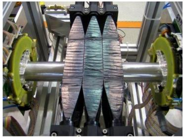
LUMI GEM detector Dafne (LNF) luminometer
