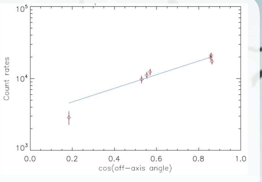
X-axis shows the cosines of det-to-source angles (angles between the detector's zenith and SGR 1935) less than 90°. Y-axis shows the peak count rates of corresponding detectors in log scale. Linear fit results indicate that the burst is in the direction of SGR 1935.
