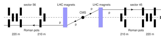
Schematic diagram of CMS-TOTEM configuration during the common run.
