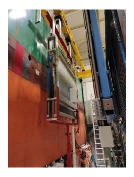
The PA05 chamber with the new iFTDC & CMAD based FEs has been instrumented
