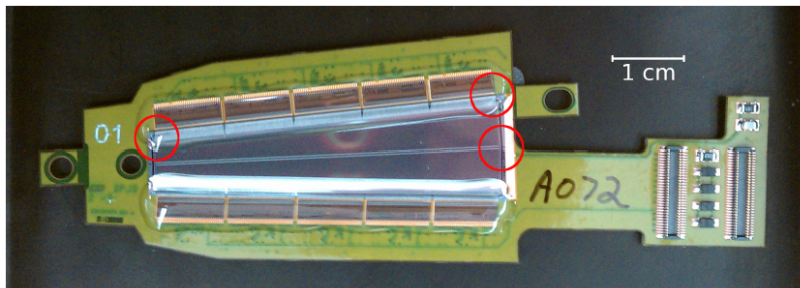
Figure 3: (color online) A completed FVTX small wedge, with sensor facing up. Note the center line dividing the two halves of the sensor and rows of FPHX chips along the sensor edges.
