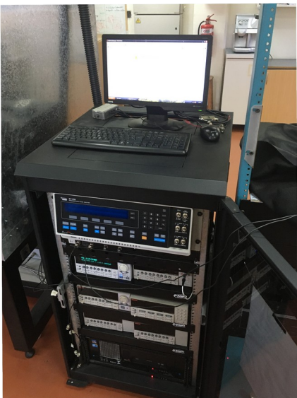
Darkcurrent measurement using SMU & Prove Station
