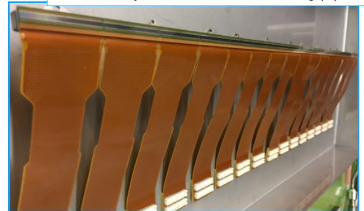
SiPM arrays mounted on the cooling pipe
