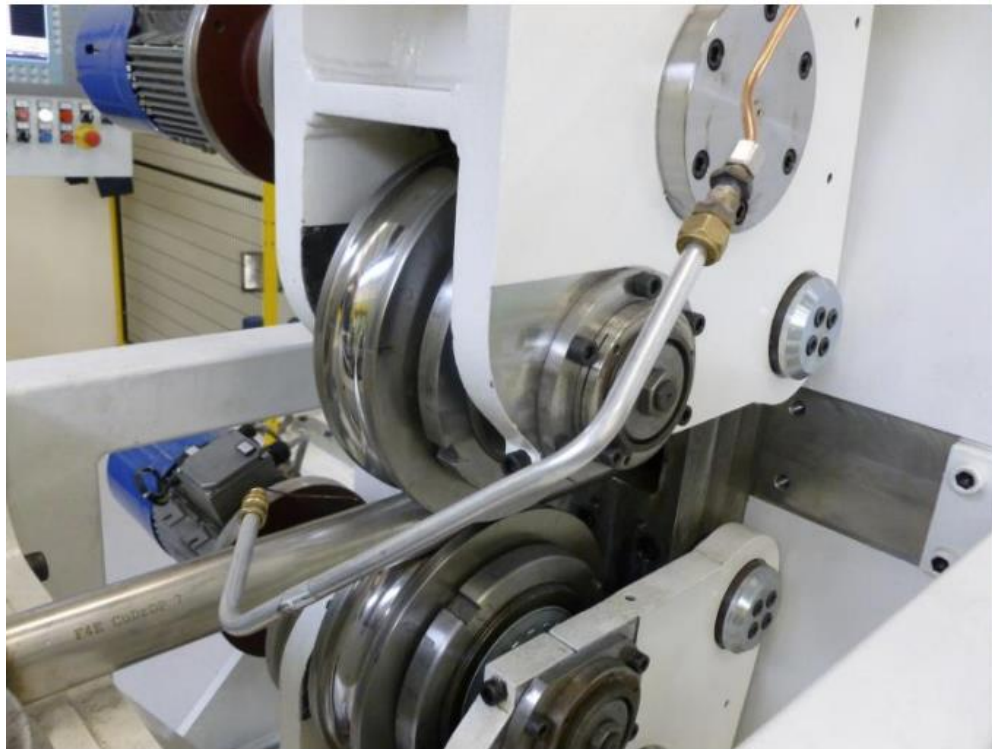
Second pair of compaction rollers
