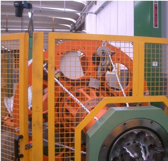
Final TF cable formation
