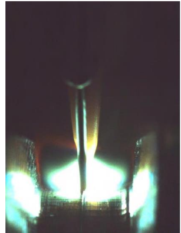
Figure 7b. electrode and filler wire during the very first pass
