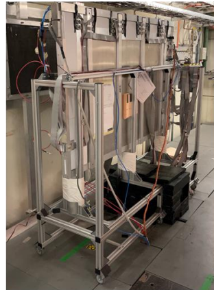
Performance measurement for ATLAS RPC BIS78 chamber inc. readout system, in presence of HL-LHC radiation background
